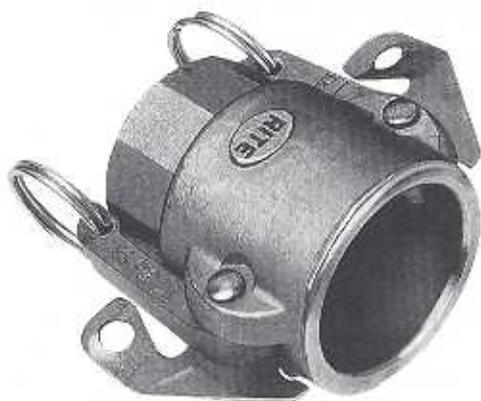
The **Anti-Vibration Spring** (Figure 1) clamps the handles in position. The spring remains attached to one of the handles when open so it cannot be lost. This lock is easily field retrofit to existing couplers. Just remove the finger ring, slide the spring on and reinstall the ring. A secondary motion is required to place the Spring in lock position.
